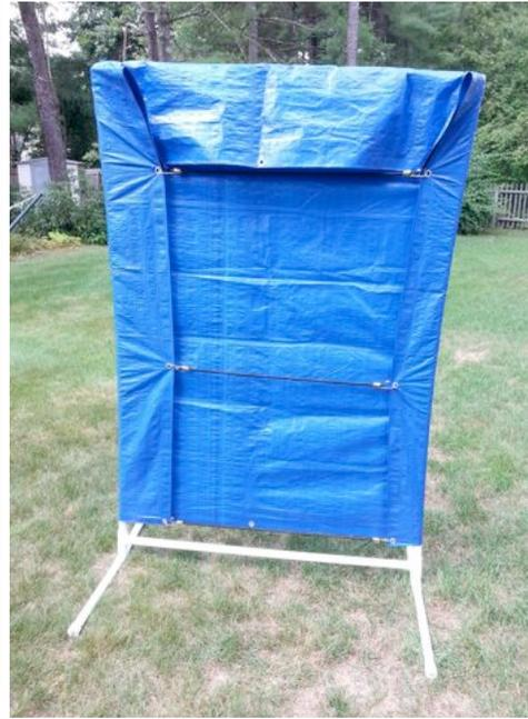
**The light shield was made from a tarp with dimensions slightly larger than the frame (in this case, 7 X 5½ feet). After draping the tarp over the frame, I secured it with three 30-inch bungee cords, inserting the hooks at the end of each cord through grommet holes in the tarp.**
