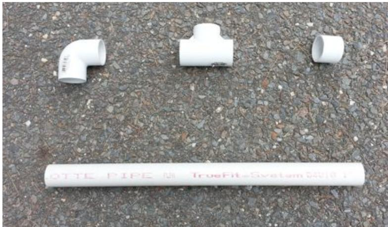
Because portability was a critical factor, I chose to work with 1-inch diameter PVC plumber's pipe and non-threaded "slip-in" fittings (90° elbows, tees, and end caps).
