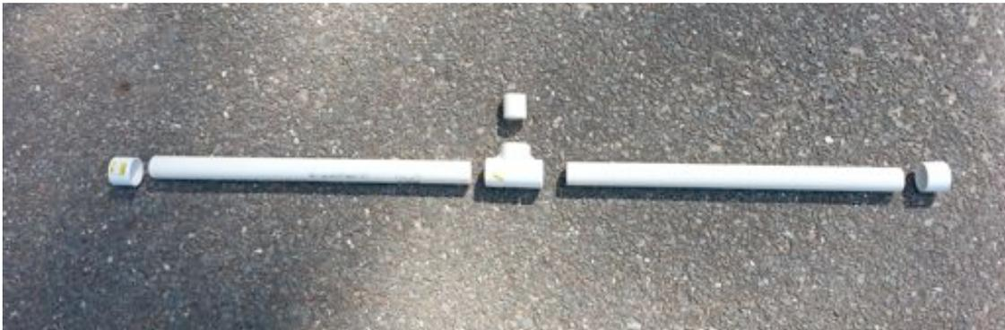
Each of the support struts was made up of two 2-foot sections of pipe joined by a tee and bracketed with end caps. A 2-inch piece of pipe was fitted into the top of the tee. This would connect the strut to the tee at the bottom of the frame.
