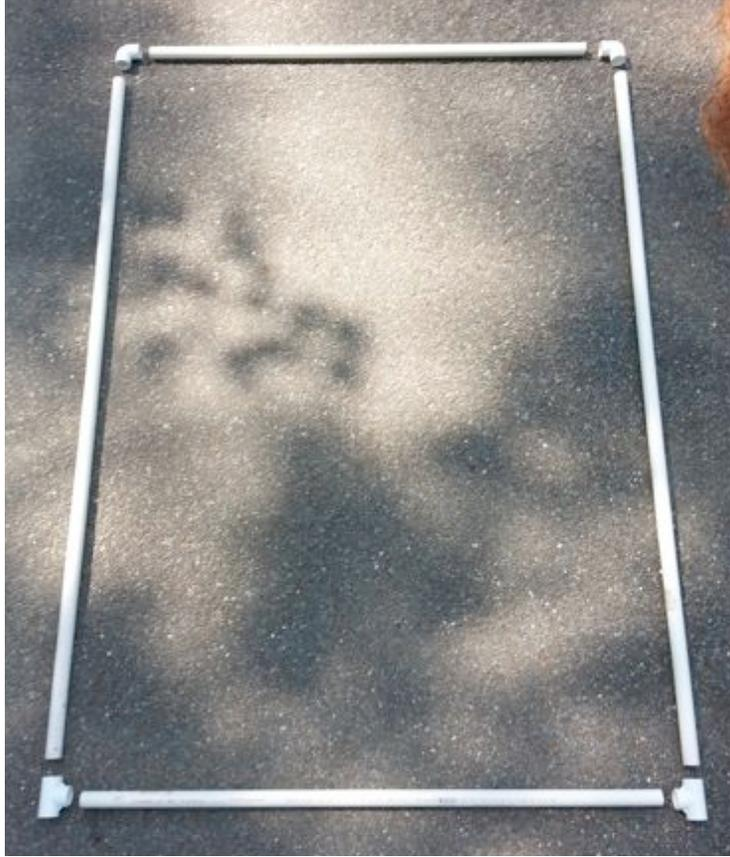
The frame was comprised of two 6-foot sections of pipe for the sides and two 4-foot sections of pipe for the top and bottom, connected at the top by 90° elbows and at the bottom by tees.
