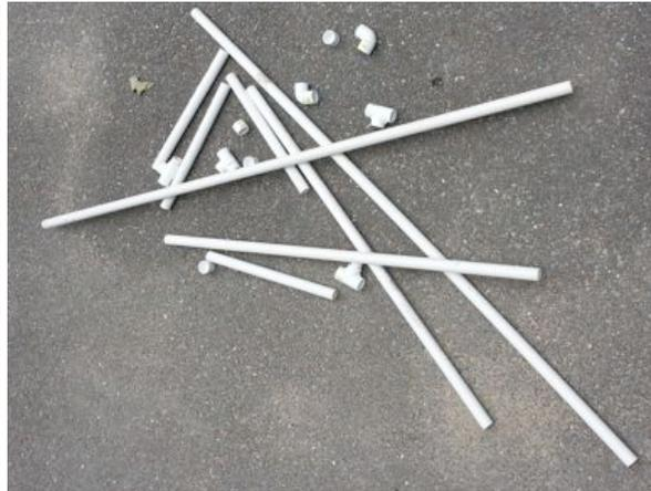
**The disassembled frame consists of 20 pieces. To avoid the risk of arriving at a star party minus a few key pieces I glued the elements (6-foot pipe, elbow, and tee) comprising each of the sides of the frame, as well as the component parts of each support strut.**
