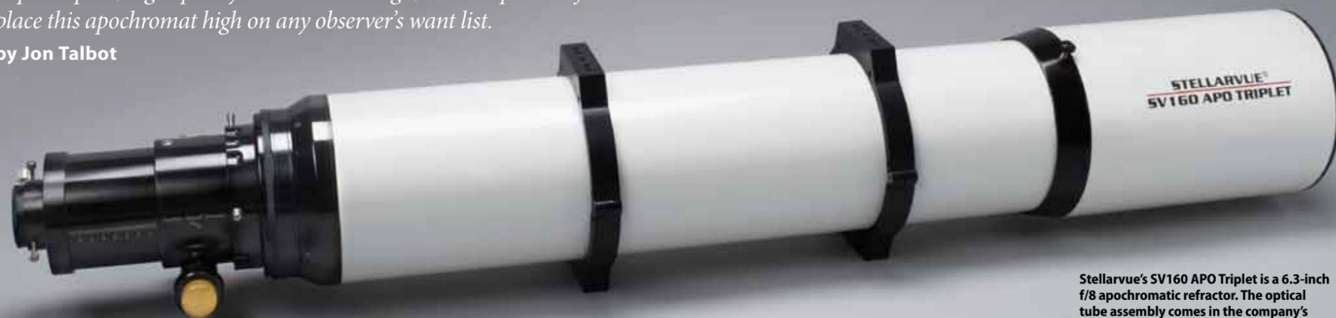
Stellarvue's SV160 APO Triplet is a 6.3-inch f/8 apochromatic refractor. The optical tube assembly comes in the company's "Stardust White" finish and has a retracting dew shield. ASTRONOMY: WILLIAM ZUBACK
