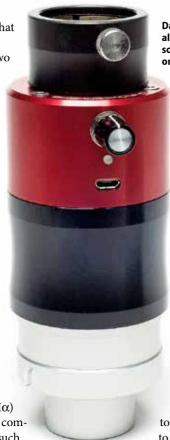
Daystar's Quark is a Hydrogen-alpha filter that fits into your telescope's focuser. The unit weighs only 13.9 ounces (394 grams).
