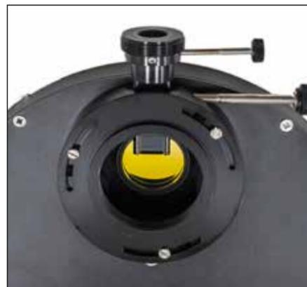
The optional off-axis guider includes a pick-off mirror that captures light through the same optics the CCD camera uses. **TONY HALLAS**
